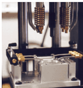
Unique Post Cooling Feature for tight stakes and faster assembly
